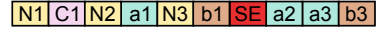
Figure 11: The hypothetical interleaving scheme for child descriptor entries and lookup entries. Illustrated is a span with three non-leaf voxels N1–N3. All boxes correspond to 32 bits. Only the first voxel has a contour lookup entry C1. Attachment lookup entries a1–a3 and b1,b3 are stored in an unintuitive but efficient way on both sides of span entry field SE. See text for discussion.
