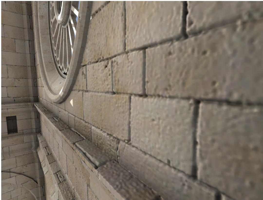
Figure 25: SIBENIK-D represented as voxels with high-resolution surface displacement and rendered with precomputed ambient occlusion and a single shadow ray per primary ray. Four samples per pixel antialiasing was used with a reconstruction filter that uses 12 samples, including 8 from neighboring pixels. 13 octree levels could be fit in memory, corresponding to voxel spacing of about 5mm.
